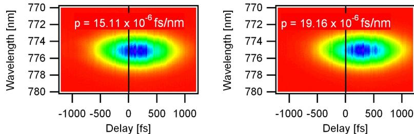
Fig. 5. GRENOUILLE traces for pulses with different amount of pulse-front tilt. The shift of the trace reveals and measures the pulse-front tilt. Note that these traces are not centered at zero delay, and the trace with greater pulse-front tilt has greater displacement from zero delay, as expected.
