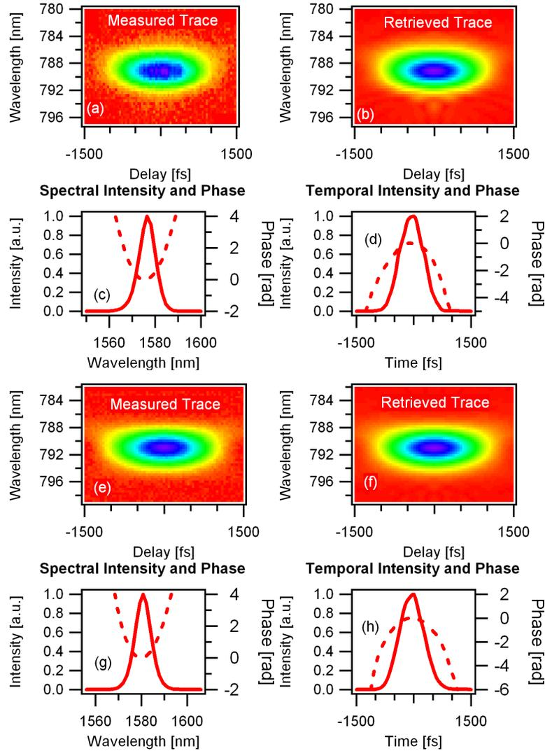
Fig. 3. Tests of our 1.5- $\mu\text{m}$  GRENOUILLE: (a) measured GRENOUILLE trace; (b) retrieved GRENOUILLE trace (FROG error:0.0055); (c-d) retrieved temporal and spectral intensity and phase (the retrieved pulse width is 779 fs and the bandwidth is 8.2 nm); (e) measured multi-shot FROG trace; (f) retrieved multi-shot FROG trace (FROG error:0.0023); (g-h) retrieved temporal and spectral intensity and phase (the retrieved pulse width is 765 fs and the bandwidth is 8.1 nm).
