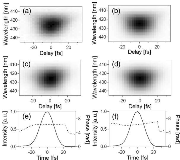
Fig. 3. Comparisons of short-pulse GRENOUILLE and multishot FROG measurements: (a) measured GRENOUILLE trace, (b) measured multishot FROG trace, (c) retrieved GRENOUILLE trace (FROG error of 0.00497), (d) retrieved multishot FROG trace (FROG error of 0.00482), (e) retrieved intensity and phase versus time for GRENOUILLE measurements (temporal pulse width of 19.73 fs FWHM), (f) retrieved intensity and phase versus time for multishot FROG measurements (temporal pulse width of 19.41 fs FWHM).
