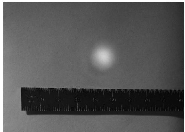
Fig. 2. Spatial profile of the continuum from the bulk fused silica using an  $\sim 5 \mu\text{J}$  pulse energy. Slight color variations (intensity variations in gray scale) occurred in this beam, so only  $3 \mu\text{J}$  was used in order to minimize the spatial variations.
