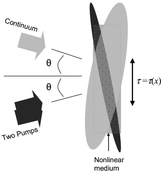
Fig. 3. Schematic of three pulses [two pumps (black) and a continuum (gray)] for a single-shot TG XFROG geometry. The continuum and two pumps cross at an angle  $\theta$  (13.5 deg), mapping delay onto the transverse position. The two pumps are overlapped in time and space and form a transient grating in the nonlinear medium. The continuum is diffracted by the transient grating.
