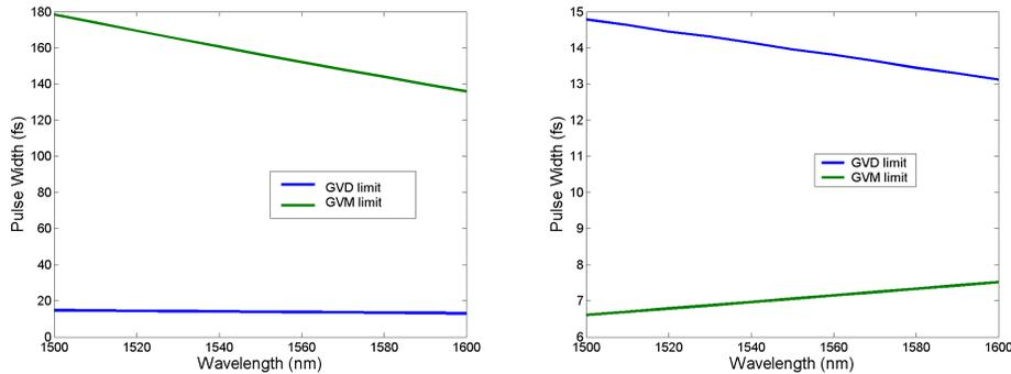
Fig.2. The theoretical shortest pulses satisfying the limits imposed by GVD and GVM, for a 1-mm-thick  $\text{LiNbO}_3$  crystal for an undithered crystal (left) and for a dithered crystal with a  $10^\circ$  scan range (right). Note that angle dithering relaxes phase-matching-bandwidth constraint, leaving the GVD constraint unchanged.
