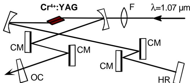
Fig. 1. The Cr<sup>4+</sup>:YAG laser setup. The mode-locking is achieved by a KLM mechanism with a prismless dispersion compensation. CM: chirped mirrors.
