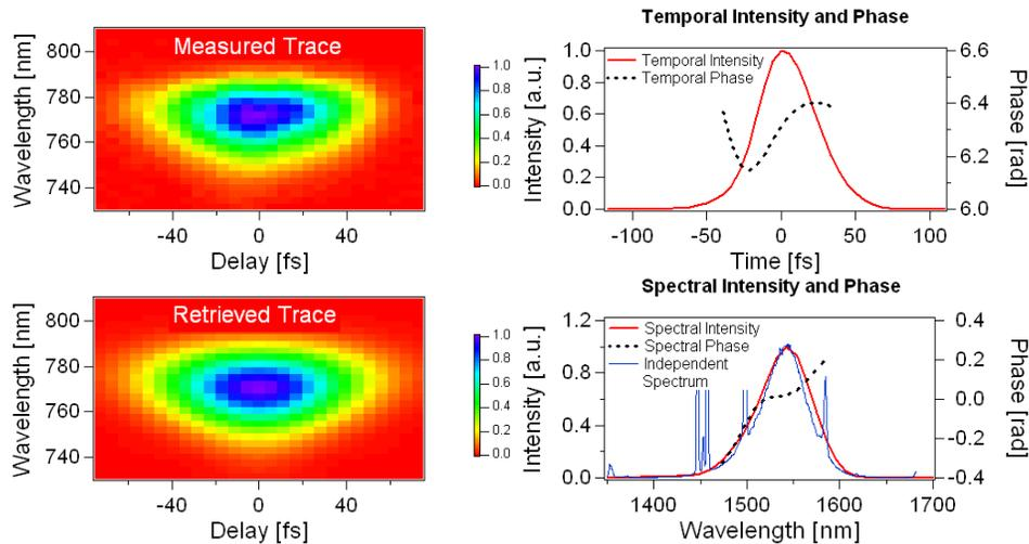
Fig. 5 FROG measurements of the intensity and phase of Cr<sup>4+</sup>:YAG laser output pulses. The retrieved pulse width is 46.6fs (FWHM). The narrow spikes in the independently measured spectrum are the cw component and sidebands originating from the higher-order dispersion inside the cavity.
