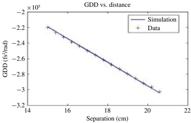
Fig. 6. GDD variation with corner cube separation.
